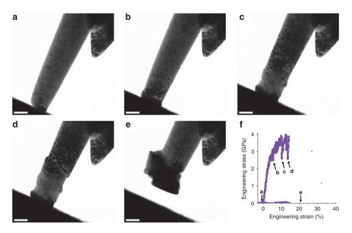
**Figure 2** | **Mechanical annealing during the** *in situ* **nanocompression test of a typical Mo nanopillar.** Bright-field TEM images of the diameter D = 142 nm pillar before (**a**) and after (**e**) the *in situ* compression test. (**b**), (**c**), (**d**) and (**e**) correspond to the marked points in the engineering stress versus strain curve in (**f**). The scale bar in each figure represents 100 nm. See also the recorded video in Supplementary Movie 1.
