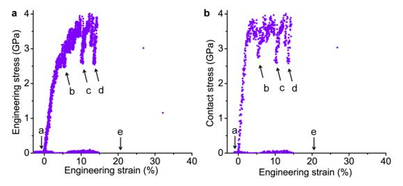
Supplementary Figure S1. Stress-strain curves for FIBed Mo pillars with diameter of 142 nm. (a) Engineering stress (force divided by a fixed cross sectional area) vs. Engineering strain (b) Contact stress (instantaneous force divided by the instantaneous contact area) vs. Engineering strain. Supplementary Figure S1a is reproduced from Figure 2f in the paper.
