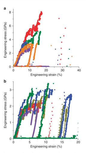
Figure 3 | Representative engineering stress-strain curves of Mo nanopillars. (a) Diameter D < 200 nm, including 80 nm (red), 120 nm (green), 165 nm (blue), 172 nm (orange) and 185 nm (purple). (b) Diameter D > 200 nm, including 268 nm (green), 369 nm (blue), 463 nm (yellow), 607 nm (red), and 1,200 nm (purple).
