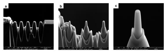
Supplementary Figure S3. Sequential FIB micromachining to obtain nano-sized pillars. (a) Rough machining. (b) Fine processing. (c) Superfine processing.
