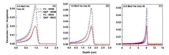
**Figure 4.** Comparison of IM3D results with SRIM predictions for vacancy depth-distributions predicted by FC and QKP methods in bulk Ni, under irradiation by  $10^5$  He<sup>+</sup> ions with different energies of (a) 0.5 MeV, (b) 1.0 MeV and (c) 5.0 MeV and normal incidence at the center point of the target.
