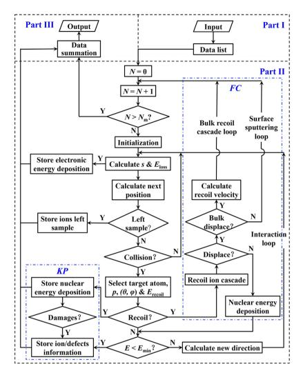
Figure 1. IM3D program flowchart showing ion tracking and defect generation methods.
