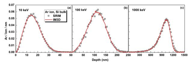
**Figure 3.** Comparison of IM3D results with SRIM predictions for Ar ion depth-distributions in Si bulk, under a total of 10<sup>5</sup> Ar ions implantation with different energies of (a) 10 keV, (b) 100 keV and (c) 1000 keV and normal incidence at the center point of the target.
