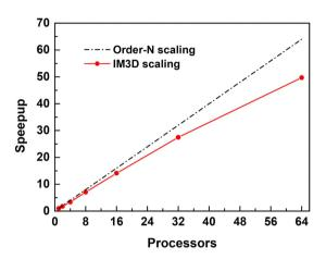
Figure 6. Wall clock scaling of IM3D with multi-processors running Message Passing Interface (MPI), for the system of a 305 nm ZrO<sub>2</sub> film on Si under a total of 10<sup>5</sup> Au ion irradiation with ion energies of 2.0 MeV.
