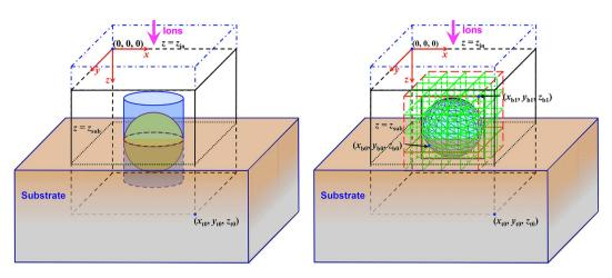
Figure 2. CSG (left) and FETM (right) geometric models and their corresponding coordinate systems.
