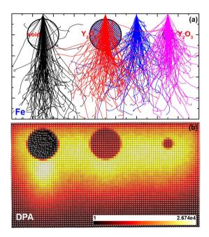
**Figure 8.** The (a) ion trajectories and (b) DPA distribution cross-section for pure iron with a void (30 nm) and two  $Y_2O_3$  nanoparticles (30 nm and 10 nm) of different sizes under 150 keV Fe ion irradiation with a normal-incidence beam.
