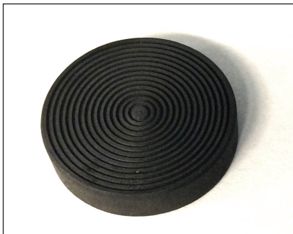
Fig. 1 — A graphite MPG-6 sample with the circular notch pattern.
