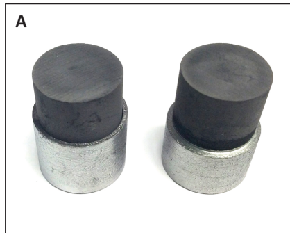
Fig. 2 — A — The samples before and after machining treatment; B — assembly for the mechanical shear tests.
