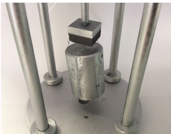
Fig. 9 — Equipment for separating the brazed joints under the load at high temperature.
