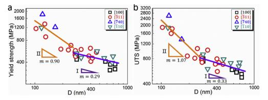
**Fig. 3.** The variation of yield strength (**a**) and UTS (**b**) of nanoscale Al-4Cu vary with the sample sizes. Both yield strength and UTS are not sensitive to loading orientations. Two size dependent stages can be divided at D = 250 nm according to the log-log plots.
