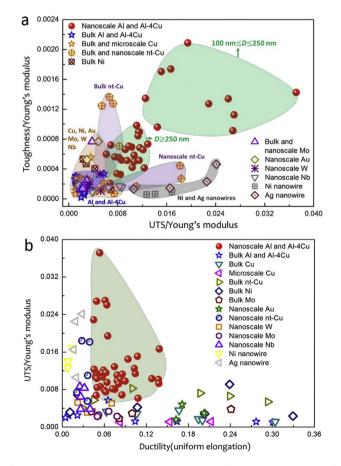
**Fig. 7.** Ashby map showing the toughness/Young's modulus versus ultimate tensile strength (UTS)/Young's modulus (**a**) and ultimate tensile strength (UTS)/Young's modulus versus ductility (**b**) plot of nanoscale Al and Al-4Cu and in comparison with other bulk or nanoscale metals [37–48]. The nanoscale Al-4Cu alloys have the unprecedented combination of toughness and UTS or UTS and ductility. The toughness is measured from the area covered by the true stress-strain curves.
