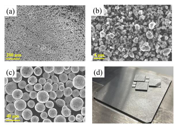
Fig. 10. (a) 420 SS powders for 3D printing, (b) Ball-milled <sup>10</sup>B particles, (c) <sup>10</sup>B doped 420 SS composite powders, and (d) 3D printed <sup>10</sup>B doped SS samples via lase powder bed fusion.
