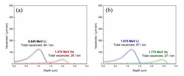
**Fig. 3.** SRIM-calculated vacancies production induced in tungsten (a) by 94% of  ${}^{10}B(n, \alpha)^7Li$  reactions (b) by 6% of  ${}^{10}B(n, \alpha)^7Li$  reactions.
