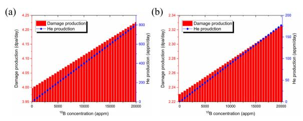
Fig. 8. Radiation damage production and helium production of iron doped with <sup>10</sup>B and <sup>235</sup>U (a) neutron irradiation with 9700 appm <sup>235</sup>U at HFIR (b) neutron irradiation with 26,000 appm <sup>235</sup>U at MITR.
