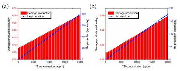
Fig. 7. Radiation damage production and helium production of iron doped with various <sup>10</sup>B (a) neutron irradiation at HFIR (the half-life of burnt <sup>10</sup>B was ~0.9 days) (b) neutron irradiation at MITR (the half-life of burnt <sup>10</sup>B was ~61.4 days).
