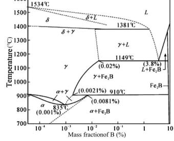
Fig. 6. Phase diagram of Fe-B [32] (taken with permission from the publisher).
