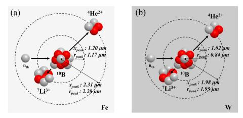
**Fig. 4.** Peak damage region of 1D ( $x_{\text{peak}}$ ) and 3D ( $r_{\text{peak}}$ ) geometry induced by <sup>10</sup>B ( $n, \alpha$ )<sup>7</sup>Li reactions in (a) iron (b) tungsten.
