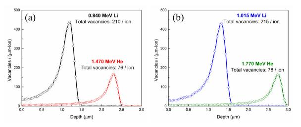
Fig. 2. SRIM-calculated vacancies production induced in iron (a) by 94% of  ${}^{10}B(n, \alpha)^7Li$  reactions (b) by 6% of  ${}^{10}B(n, \alpha)^7Li$  reactions.
