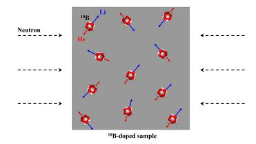
**Fig. 1.** Schematic illustration of <sup>10</sup>B doping methodology to simulate helium production and dpa accumulation (Not to scale). Note that the outgoing Li (blue) and He (red) ions have spherically random momenta, unlike the energetic ions produced by ion accelerators, thus mitigating potential polarization artifacts [29].
